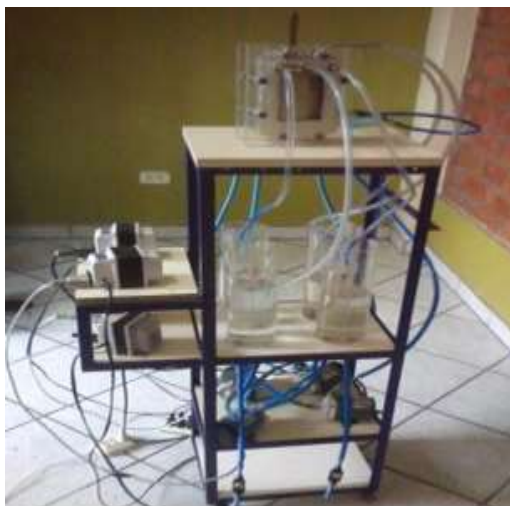
Figure 3. Bipolar Electro dialysis Pilot plant for production of hydrochloric acid through wastewater regeneration of ion exchange resins
