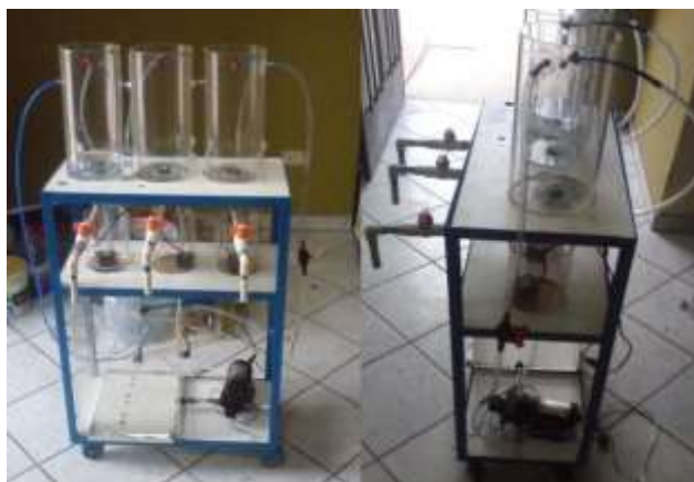
Figure 2. pre-treatment equipment for water of resin regeneration for the production of hydrochloric acid
